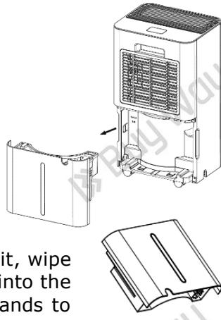
Turn the water tank upside down and empty it, wipe its exterior to ensure it is dry and reinsert it into the dehumidifier and slightly push it with both hands to ensure that it is securely positioned into place.
