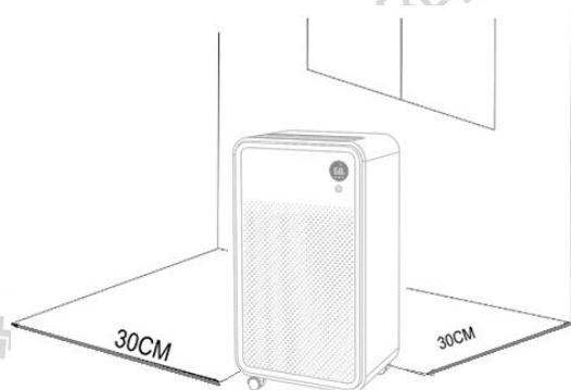
For the most effective use, run your dehumidifier with doors and windows kept closed. Please note that the unit should not be placed directly against a radiator, or gas stove or fire place or any other heat source.
